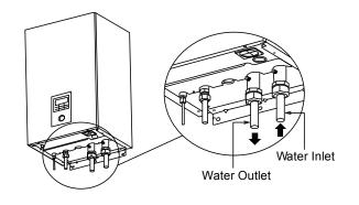
Do not over tighten, over tightening cause water leakage.
