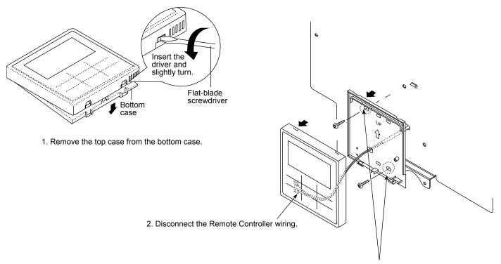
3. Remove 2 screws then take out the bottom case.
