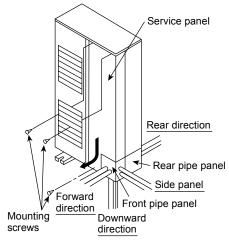
Close the tube joining area with putty heat insulator (local supply) without any gap as shown in right figure. (To prevent insects or small animal entering.)
