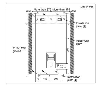
The centre of installation plate should be at more than 375 mm at right and left of the wall.
