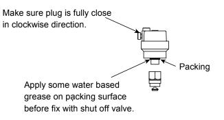
During reinstall Flow Sensor
