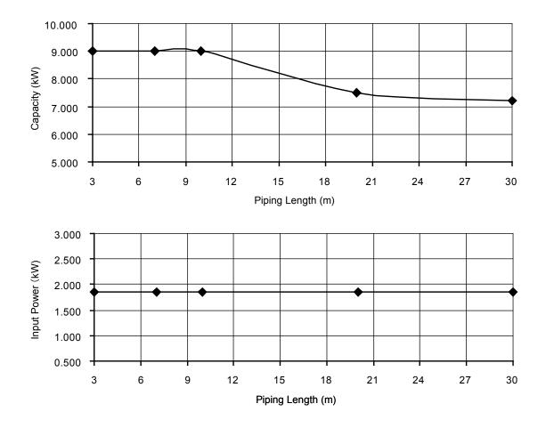
**Cooling Characteristics at Different Piping Length**
