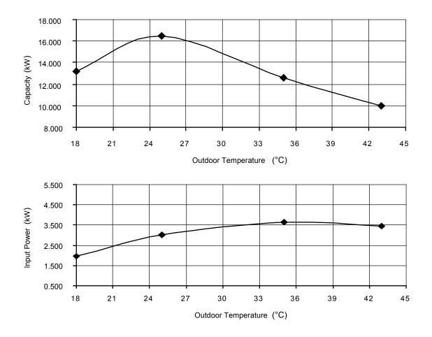
Cooling Characteristics at Different Outdoor Air Temperature
