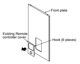
Press from front to fix the Remote controller cover
