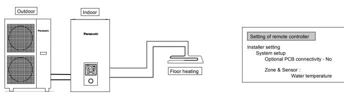
Connect floor heating or radiator directly to the indoor unit. Remote controller is installed on indoor unit. This is the basic form of the most simple system.
