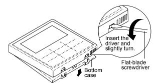
Remove the wiring between Remote controller and Indoor Unit terminal. Remove the bottom case from the Control board cover by loosening the screws. (3 pieces)
